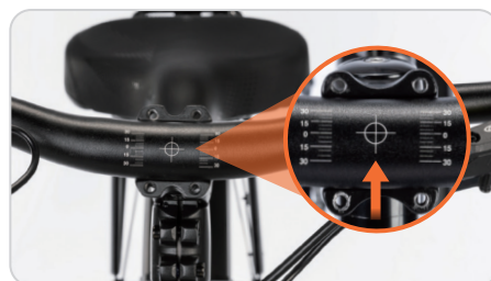
6. Install the handlebar and align the center mark to the middle.
