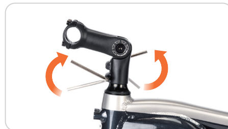
3. Lightly tighten screws A and B to hold it in place for later adjustment.
